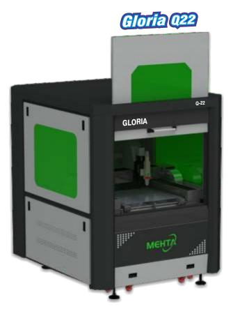
Q22 Is Special For High Precision Machinery Parts And Microelectronics And Jewelry Industries. Q22 Is Very High Speed And Higher Precision Professional Machine For Cutting Thin Metal Sheet Like Stainless Steel, M.S., Carbon Steel, Galvanized Steel, Copper, Aluminum, Brass, Gold, Silver Etc.
