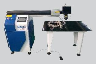
This machine used for the welding of LED illuminated billboard, exterior/interior sign, branding, door plate that made of aluminum, S/S, iron, galvanized sheet, titanium, brass, copper, and etc. Laser beam with high energy melts two metal sheets and combine them together without feeding any soldering materials. from any aspect, laser welding is the best solution and the greenest.
